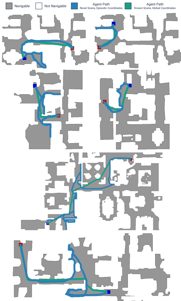
Figure A6: True state trajectory comparison. Example trajectories of an agent with true state (trained for a specific environment and using global coordinates), green line, compared to an agent trained for many environments and using episodic coordinates, blue line. The later is what we examine in this work. Notice that the agent with true state take shortest path trajectories while the agent without true state instead exhibits strong wall-following behavior.
