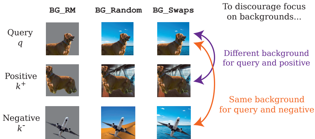
Figure 2: Schematic of different types of background augmentations. BG_RM (left) replaces backgrounds with grayscale, effectively removing any background information. BG_Random (middle) replaces backgrounds with random backgrounds, creating a random signal which is uncorrelated with the foreground. BG_Swaps (right) exploits the structure of contrastive learning to ensure that the query and the positive have the same foreground but different backgrounds, while the query and one negative have matched backgrounds. As a result, BG_Swaps makes it so that models are penalized for focusing on the background.
